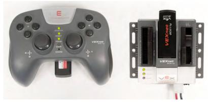
g. If the units fail to establish the VEXnet link after 30 seconds, turn them both OFF and then back ON. If they still fail to link up, refer to the Troubleshooting Flowchart in section 7.
