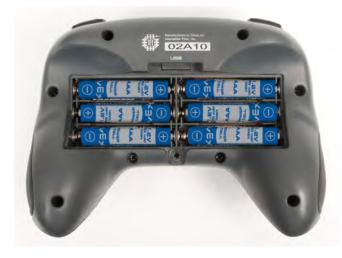
c. Reinstall the battery cover (insert the two tabs of the battery cover first along the back edge of the battery cover to aid in installation) and then tighten the cover screw. Then add the VEXnet 802.11g key as shown.
